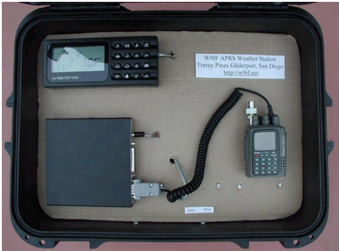
Part 4 - Figure 2. Weather station console (upper left), TNC (lower left), and two meter transceiver (right) comprise the indoor components of the system.
