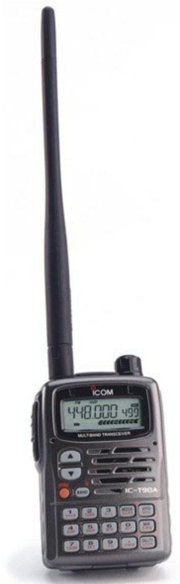
Part 2 - Figure 1. Other than size, this 2 meter amateur radio has little in common with a business radio. It provides more control and features such as a computer interface for programming. Photo courtesy of ICOM America Inc.
