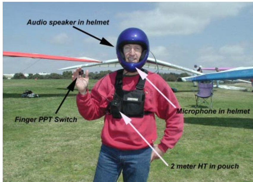
Part 1 - Figure 2. The author, ready for aeronautical mobile communication using a hands-free system for control.
